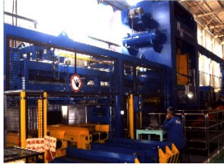
400 tons high accuracy automatic production line for stamping of stator and rotor silicon steel sheet
