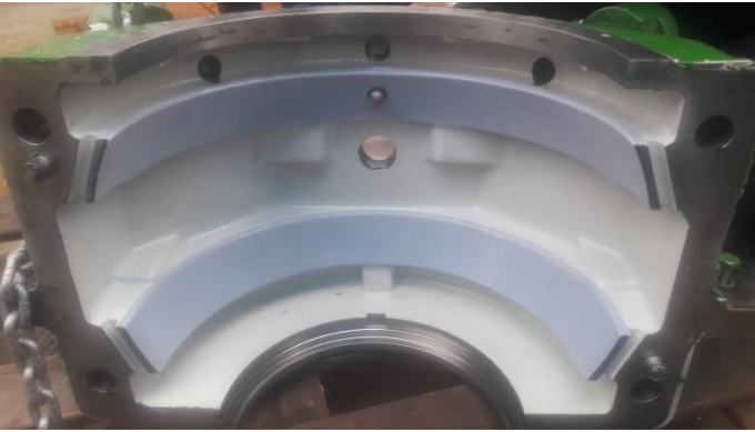
There is no problem in the upper and lower housing and inulations
