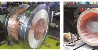
Manufacture of roller motor collectors.
