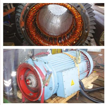
250 kW Atlas Copco compressor motor winding.
