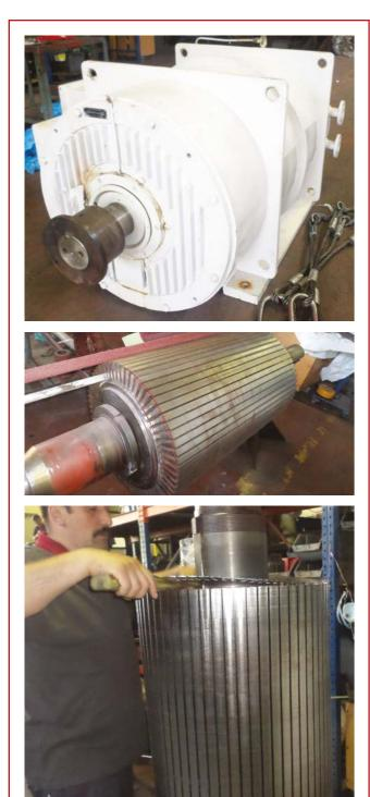
1475 kW Pump motor rotor core manufacture and rewinding.
