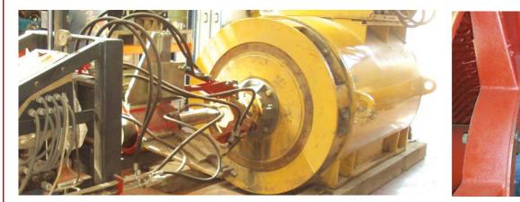
1165 KW Cogeneration generator field turnkey maintenance work.
