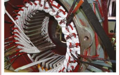
150 kW AC traction motor stator winding work.
