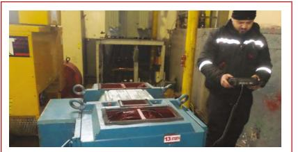
700 kW DC roller motor maintenance.
