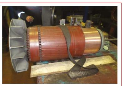
128 kW DC traction motor stator winding work.
