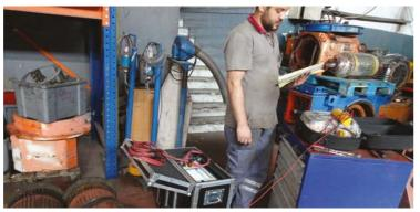
70 kW traction AC generator maintenance work.
