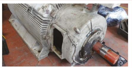
ISKI 1000 kW Pump motor maintenance and repair.
