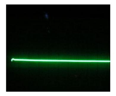
Figure 3 shows an actual winding trace indicating the presence of one or more shorted-turns:
